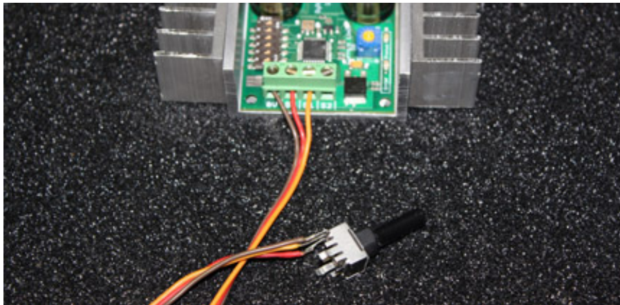
Figure 2.1: Analog input using a potentiometer powered from terminal 5V
