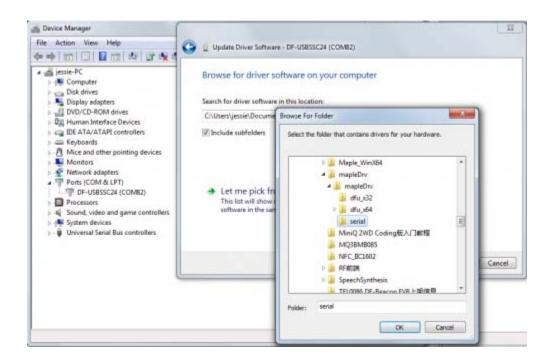
5) Reset Veyron Servo Driver 24-Channel with RET button, wait for the blue light stops flashing. At this point Windows will prompt to install the driver, too. Please manually locate the directory, select mapleDrv -->serial in the folder. Until now, the driver has been installed
