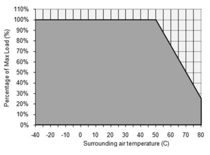
Fig. 1 De-rating for Vertical and Horizontal Mounting Orientation  $> 50^{\circ}$ C de-rate power by 2.5% / °C
