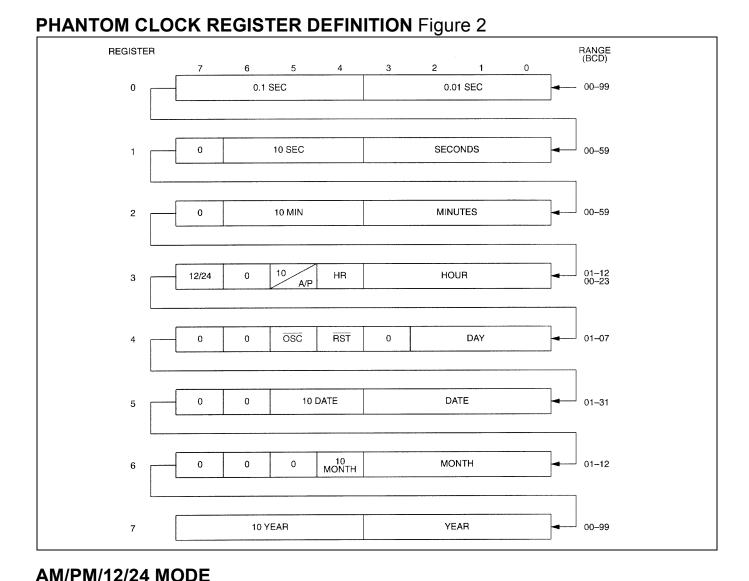
Bit 7 of the hours register is defined as the 12-hour or 24-hour mode-select bit. When high, the 12-hour mode is selected. In the 12-hour mode, bit 5 is the AM/PM bit with logic high being PM. In the 24-hour mode, bit 5 is the 20-hour bit (20–23 hours).
