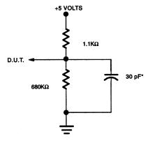
\* INCLUDING SCOPE AND JIG CAPACITANCE
