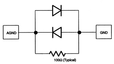
NOTE: GND and AGND must be tied to the same voltage level.
