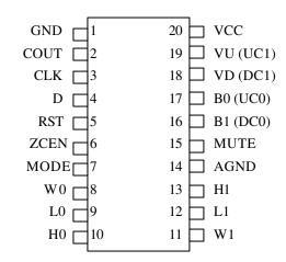
20-Pin DIP (300-mil) 20-Pin SOIC (300-mil) 20-Pin TSSOP (173-mil) See Mech. Drawings Section
