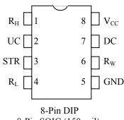
8-Pin SOIC (150-mil) 8-Pin μSOP (118-mil)
