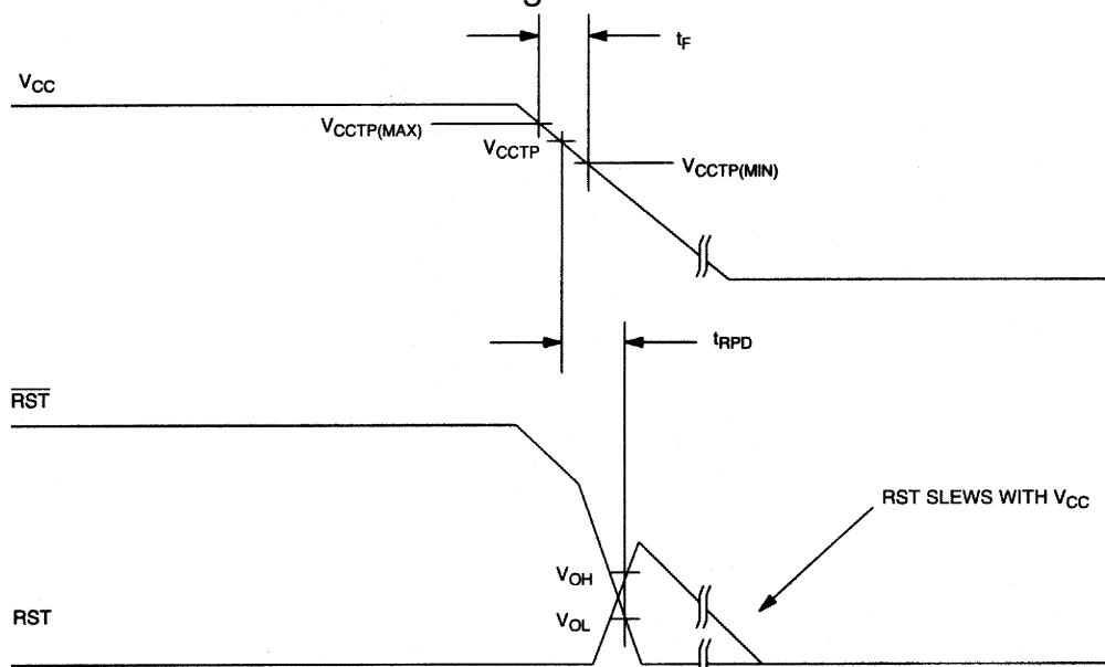
**TIMING DIAGRAM: POWER-UP** Figure 7
