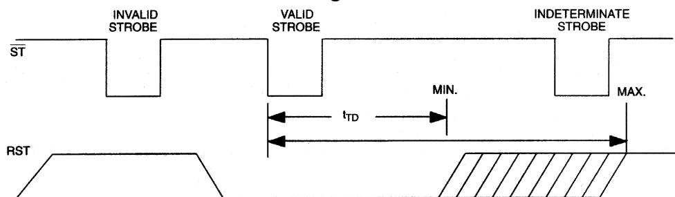
**TIMING DIAGRAM: POWER DOWN** Figure 6
