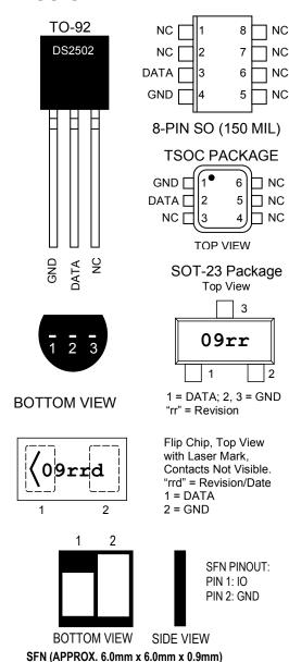
**NOTE:** THE SFN PACKAGE IS QUALIFIED FOR ELECTRO-MECHANICAL CONTACT APPLICATIONS ONLY, NOT FOR SOLDERING. FOR MORE INFORMATION, REFER TO APPLICATION NOTE 4132: ATTACHMENT METHODS FOR THE ELECTRO-MECHANICAL SFN PACKAGE.
