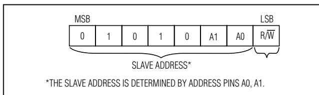
Figure 1. DS3502 Slave Address Byte
