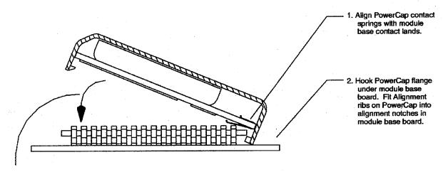
3. Push down slot side of PowerCap until it snaps onto module base.
