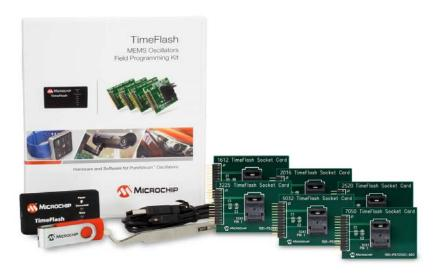
The TimeFlash programmer allows users to rapidly program Microchip's field programmable MEMS oscillator to a custom frequency in seconds, minimizing design time by enabling fast prototyping and testing. Our MEMS oscillators are available in industry standard packages that are drop-in replacements to standard crystal oscillators
