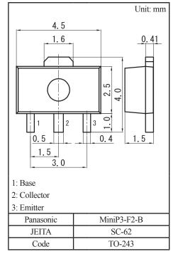
Note) Printed circuit board: Copper foil area of  $1~\rm cm^2$  or more, and the board thickness of  $1.7~\rm mm$  for the collector portion
