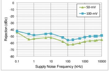
Power supply rejection ratio
