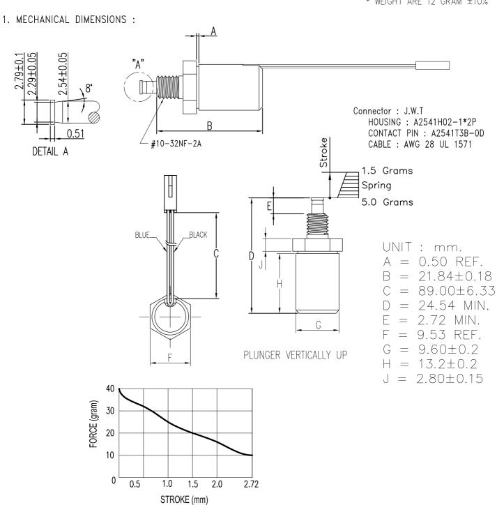
INSULATION MATERIALS: UL CONSTRUCTION, CLASS B 130°C LIFE EXPECTANCY: 100K CYCLES OPERATIONS
