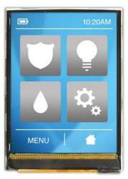
The Displaytech DT028ATFT-PTS is a display module that contains a TFT with projected capacitive touch (PCAP) technology. This 2.8 inch TFT LCD display module has 320 x 240 RGB resolution and displays 262K colors. The 5-finger multi-touch capability of this PCAP TFT allows for gesture recognition and high performance accuracy. Utilize touchscreen technology with the Displaytech DT028ATFT-PTS!
