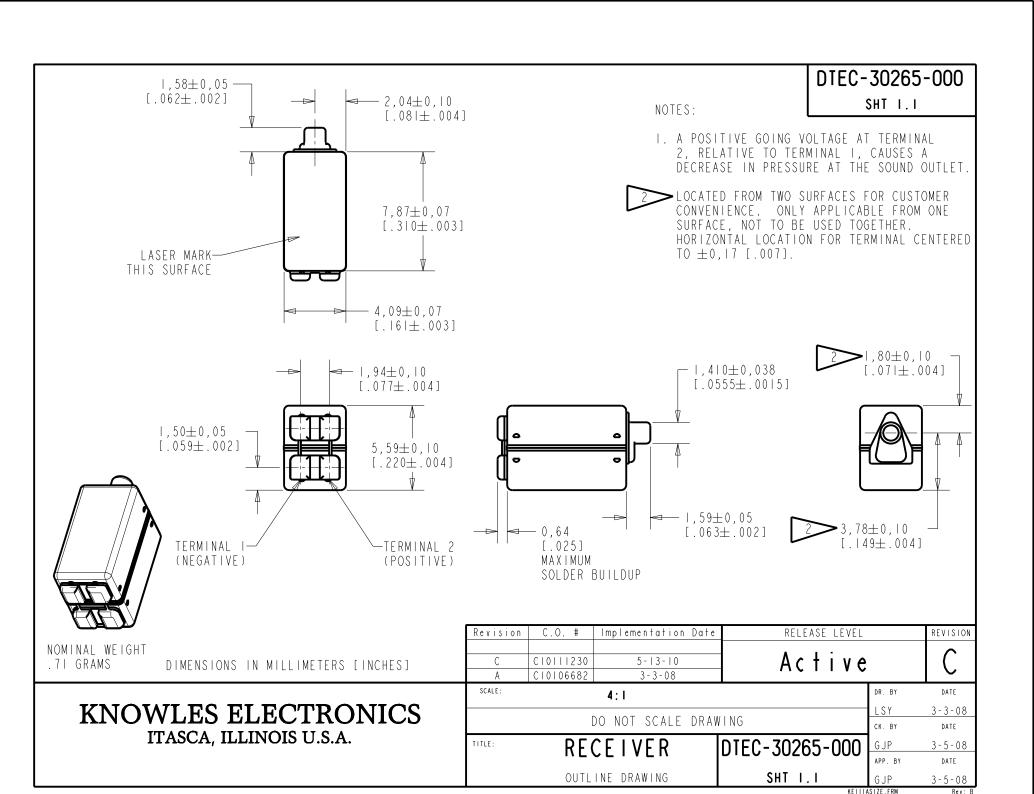
THE DTEC-30265-000 IS A PAIR OF BALANCED ARMATURE RECEIVERS INTENDED FOR USE IN BTE HEARING AIDS, AND IS THE SAME SIZE AS AN EF RECEIVER.
