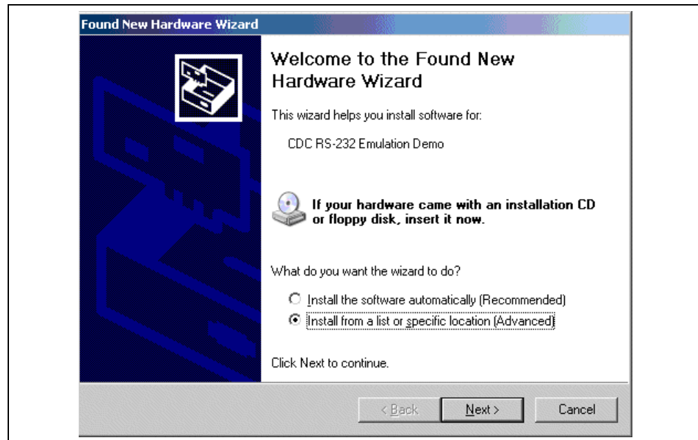
FIGURE 2-11: INSTALLING USB *.inf FILE ON PC – SCREEN 1
