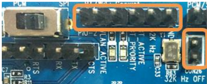
Figure 2: Pin Headers - J12 and CON26
