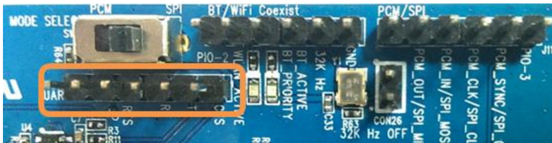
Figure 4: Pin Header J10
