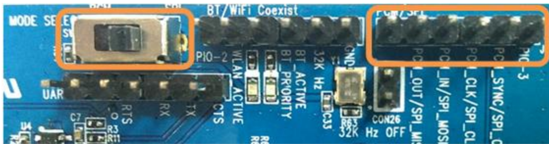
Figure 3: Pin Headers - J11 and SW5
