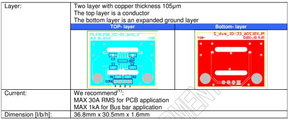
(1): The maximum current is limited by the PCB. For higher currents (> 30A), one can use an external conductor (i.e. a bus bar).
