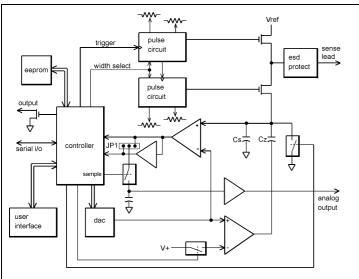
required to create a prox 'trip' for the object presented; this feature eliminates the need for sensitivity potentiometers. There are three different calibration modes to select from.
