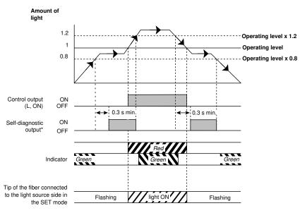
\*If the self-diagnostic output is ON when the sensing object is moving at low speed, use the E3X with an ON-delay timer circuit.
