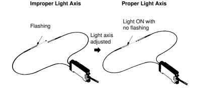
Set the mode selector to L-ON or D-ON after the light axis is adjusted.
