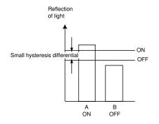
Detecting operation is not stable because zone B is within the hysteresis differential range. Reduce the sensitivity of the E3X with the sensitivity adjuster and turn off zone B.
