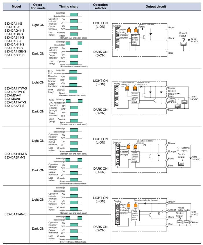
Note: The ON/OFF regions when areas settings are used with the E3X-DA□TW-S are as follows: LIGHT ON: ON when the incident level is between the thresholds for channels 1 and 2. DARK ON: OFF when the incident level is between the thresholds for channels 1 and 2.
