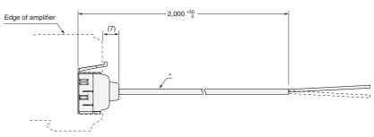
\* E3X-CN12: **2.6 dia.** cable / **1 conductor** / Standard length: 2 m (Conductor cross section: 0.2 mm² (AWG24), Insulator diameter: 1.1 mm) E3X-CN22: **4 dia.** cable / **2 conductors** / Standard length: 2 m (Conductor cross section: 0.2 mm² (AWG24), Insulator diameter: 1.1 mm)
