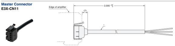
\* E3X-CN11: 4 dia, cable / 3 conductors / Standard length: 2 m (Conductor cross section: 0.2 mm<sup>2</sup> (AWG24), Insulator diameter: 1.1 mm)
