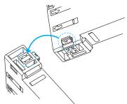
2. Remove the clip by rotating the Amplifier Unit.
