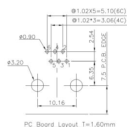
Component Side Shown Tolerance ±0.05mm
