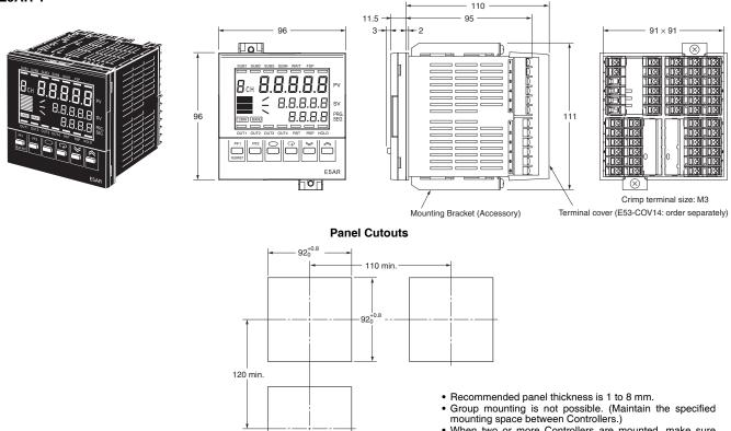
When two or more Controllers are mounted, make sure that the surrounding temperature does not exceed the allowable operating temperature specified in the specifications.
