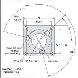
Applicable model: E6C3-A, E6C3-C Note: Three phillips screws M4 × 8 provided
