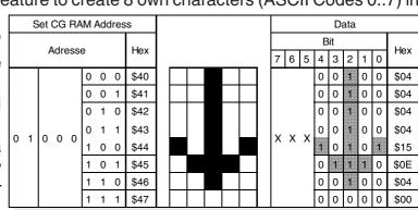
3.) The newly defined character can be used as a "normal" ASCII code (0..7); use with "DD RAM Address Set" and "Data Write".
