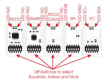
The optional adapter board EA 9777-2PE expands the Evaluation board with important interfaces: "real" RS232, RS232 CMOS, RS485, SPI and I<sup>2</sup>C.
