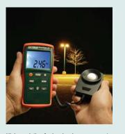
High resolution for low level measurements in places like parking lots, stairwells, and ATM machines
