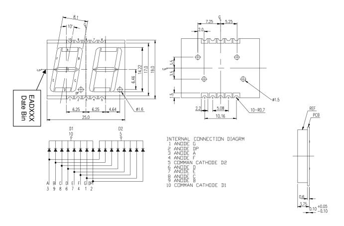
Note: Tolerances unless mentioned ±0.25mm. Unit = mm
