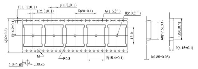
Note: Tolerances unless mentioned ±0.25mm. Unit = mm
