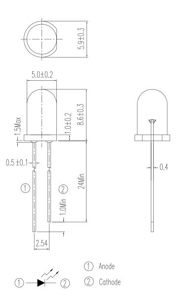
Note: Tolerances unless dimensions ±0.25mm
