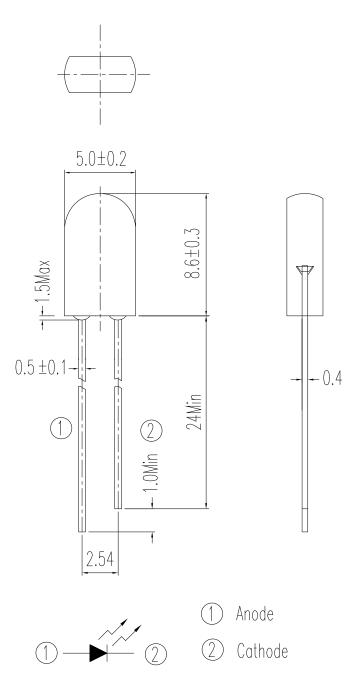
Note: Tolerances unless dimensions ±0.25mm
