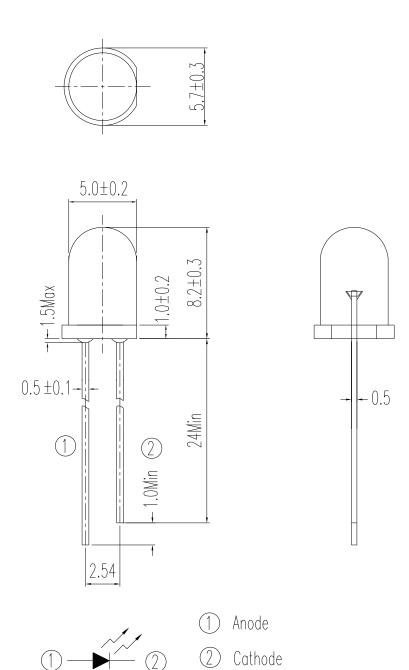
Note: Tolerances unless dimensions ±0.25mm
