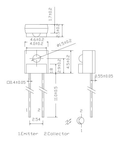
Note: Tolerances unless dimensions ±0.25mm
