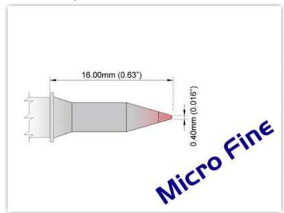
EBM7 C004 Conical 0.40mm (0.016"), Micro Fine
