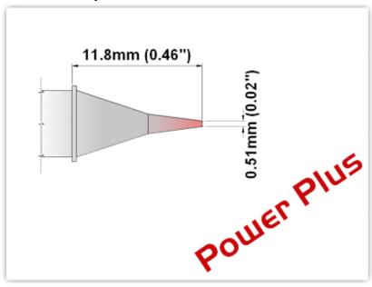
EBM7CS152H Conical Sharp 0.5mm (0.02"), Power Plus
