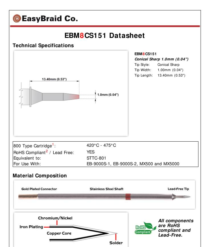
Easy Braid Co. tip cartridges will typically idle within a temperature range of +/-1.1°C. However, there is variation in idle temperature across tip geometries within an individual temperature series. Easy Braid Co. offers a wide variety of tip geometries from 0.25mm fine point tip to 5mm chisel. The length and geometry of a tip will have an influence on the tip idle temperature. To accurately measure idle temperature it will depend greatly on the measurement method,
