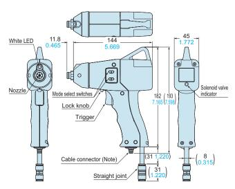
Note: An exclusive intermediate cable (oil-resistant, heat-resistant, flexible type, ø3.7 mm ø0.146 in, 2 m 6.562 ft long) is attached.
