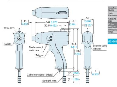
Note: An exclusive intermediate cable (oil-resistant, heat-resistant, flexible type, ø3.7 mm ø0.146 in, 2 m 6.562 ft long) is attached.
