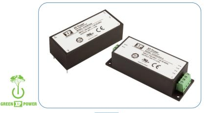
The ECE60 series of compact encapsulated AC-DC power modules are available in both PCB & chassis mount versions offering exceptional power density of  $>10W/in^3$ . Output voltages are available from 3.3 – 48 VDC and these "green power" modules offer high active mode efficiency and low no load power consumption. They also provide a peak load capability up to 130% of nominal power for up to 30s and a wide operating temperature range from -40 to +70°C.
