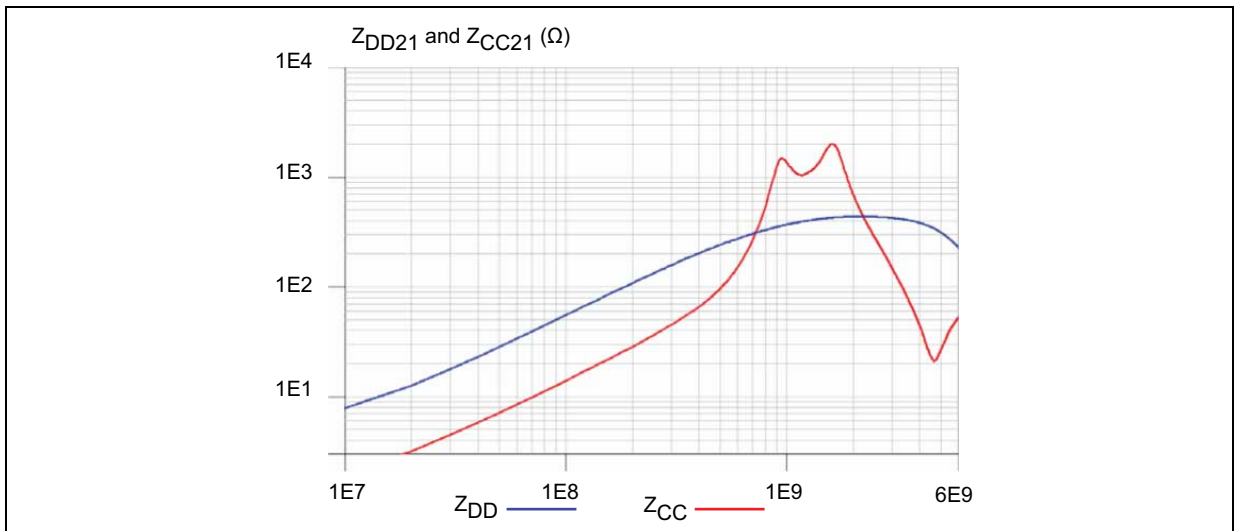
Figure 6. Differential ( Z_{DD21} ) and common mode ( Z_{CC21} ) impedance versus frequency
