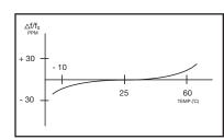
Figure 3) Frequency vs Temperature Curve
