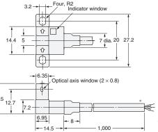
\* Vinyl-insulated round cable of 3.5 dia., 3 cores, (0.14 mm² with 1.0-dia. insulator); Standard length: 1 m
