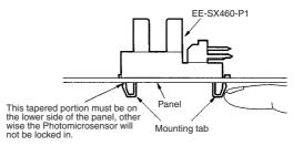
**EE-SX460-P1** Photomicrosensor (Transmissive) 145
