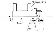
Pressed mounting holes are ideal for mounting the Photomicrosensor. When mounting the Photomicrosensor to a panel that has pressed mounting holes for the Photomicrosensor, be sure to mount the Photomicrosensor on the pressing side of the panel, otherwise it may be difficult to mount the Photomicrosensor and an insertion force of five to six kilograms may be required.
