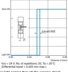
Note: The data applies to dark status. Operation may be affected by external light interference or light coming through the sensing object.
