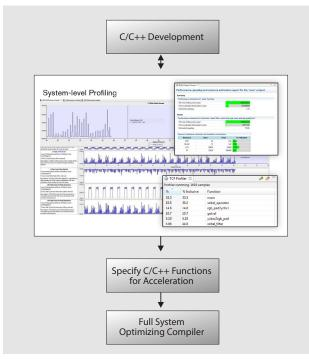
SDSoC allows users to profile their software application, using a non-intrusive profiler based on PC sampling as well as using the standard gprof profiler, to identify the function that takes up most of the time and are candidates for hardware acceleration.
