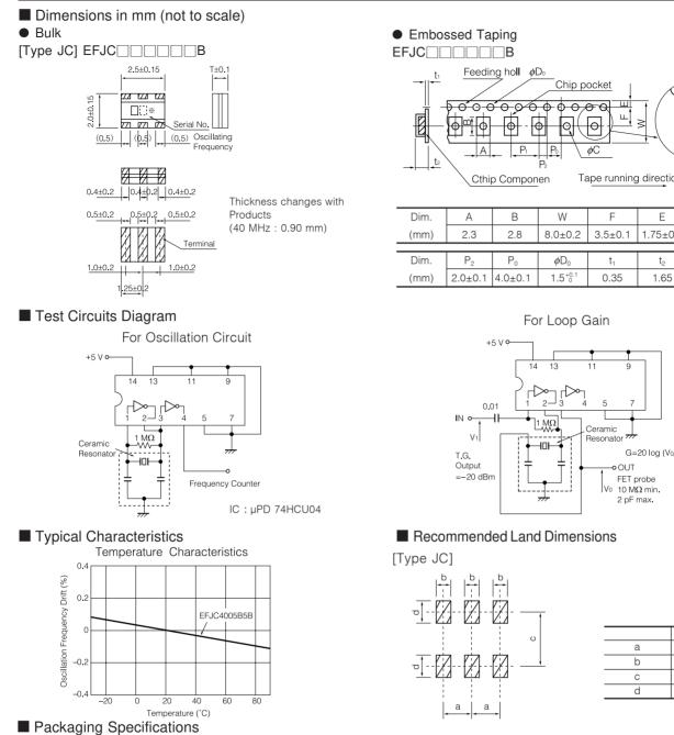
Supplied in bulk or taped & reel packing style
